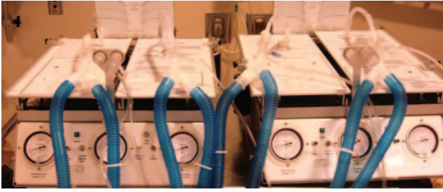
Fig. 1. Photograph of the 2 test lungs simulating 4 patients and the 4 individual circuits. Fixed orifice pneumotachographs are connected between the circuit outlet and the test lung.
